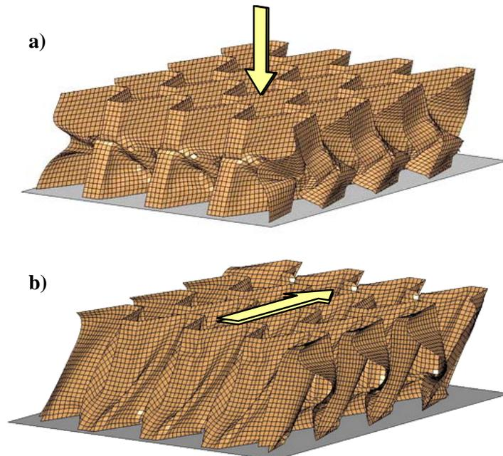
Figure 5: Folded core under a) flatwise compression and b) transverse shear load
