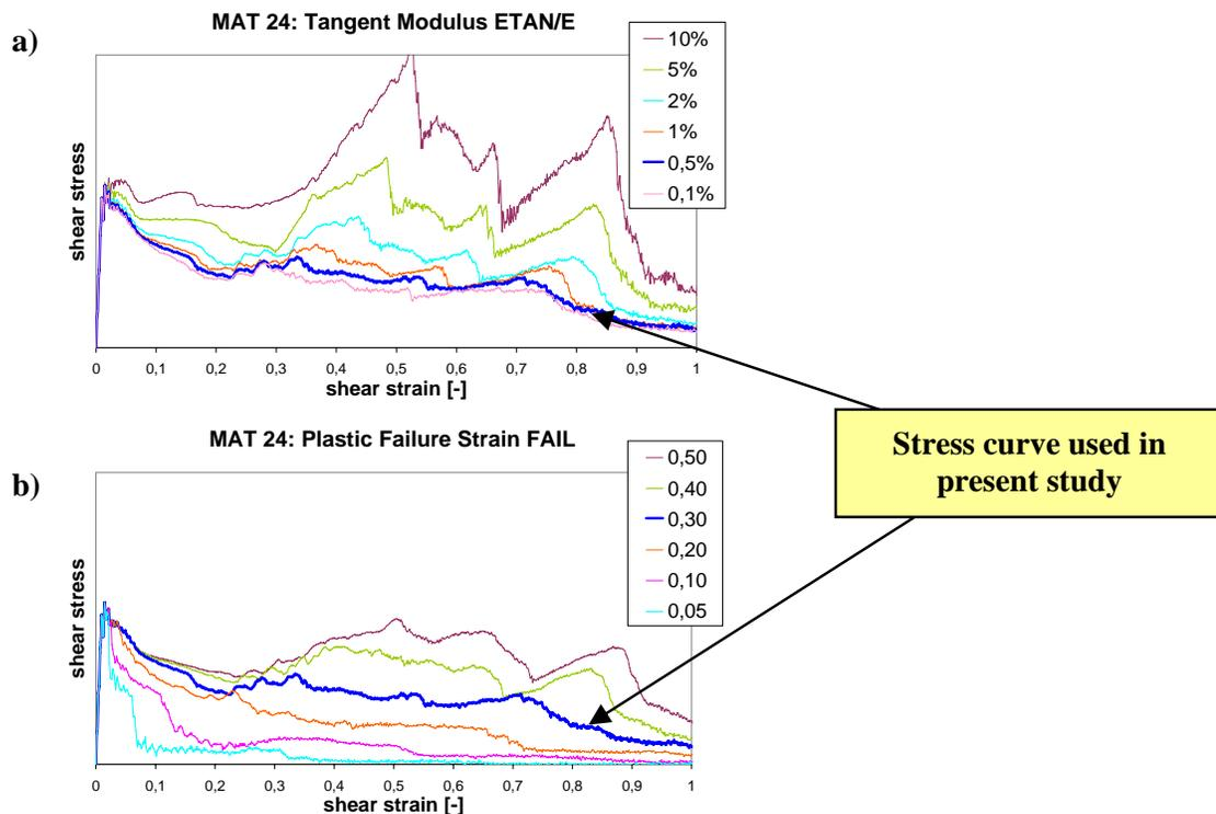
Figure 7: Influence of the parameters a) ETAN and b) FAIL in MAT 24 on the LT shear stress curve
