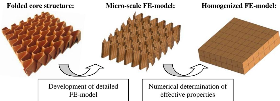
Figure 2: Approach for the numerical determination of the effective properties of folded core structures
