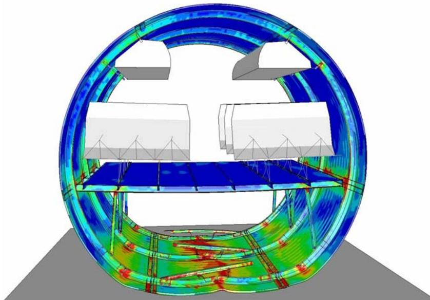
Figure 8: Drop test simulation of sandwich fuselage barrel
