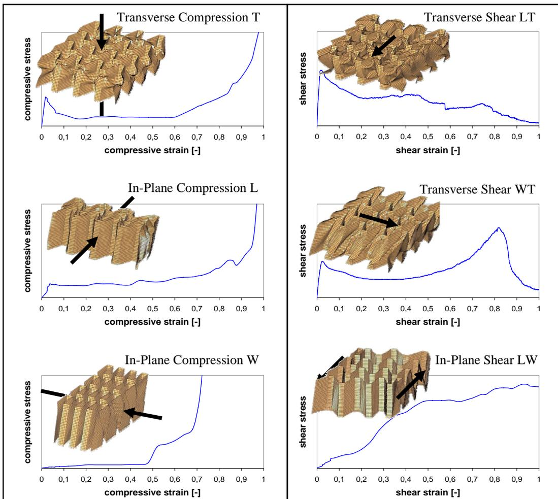
Figure 6: Qualitative stress-strain diagrams of folded core for compression and shear loads in all three material directions
