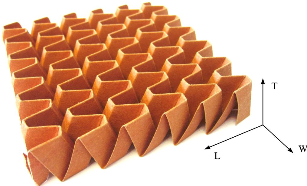
Figure 1: Folded core structure made of Kevlar<sup>®</sup> paper and its material axes
